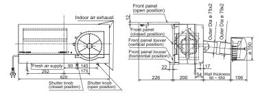
If the wall is thicker than 550mm, use the extension pipes and the pipe extension joints (separately sold parts).\*8
