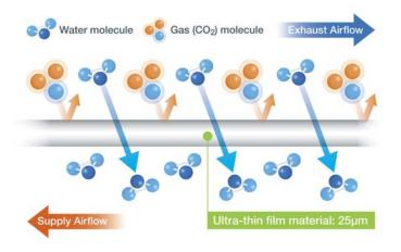
With a thickness of just 25µm, the paper used in the Lossnay core is as thin as some household aluminium foils.
